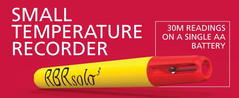
The RBRsolo<sup>3</sup> T is one of RBR's most compact, lightweight, and versatile single channel recorders. The logger offers flexible measurement schedules, standard sampling up to 2Hz (optionally up to 32Hz), large memory, extra power for extended deployments, USB-C download for large data files, and temperature accuracy of ±0.002°C.
